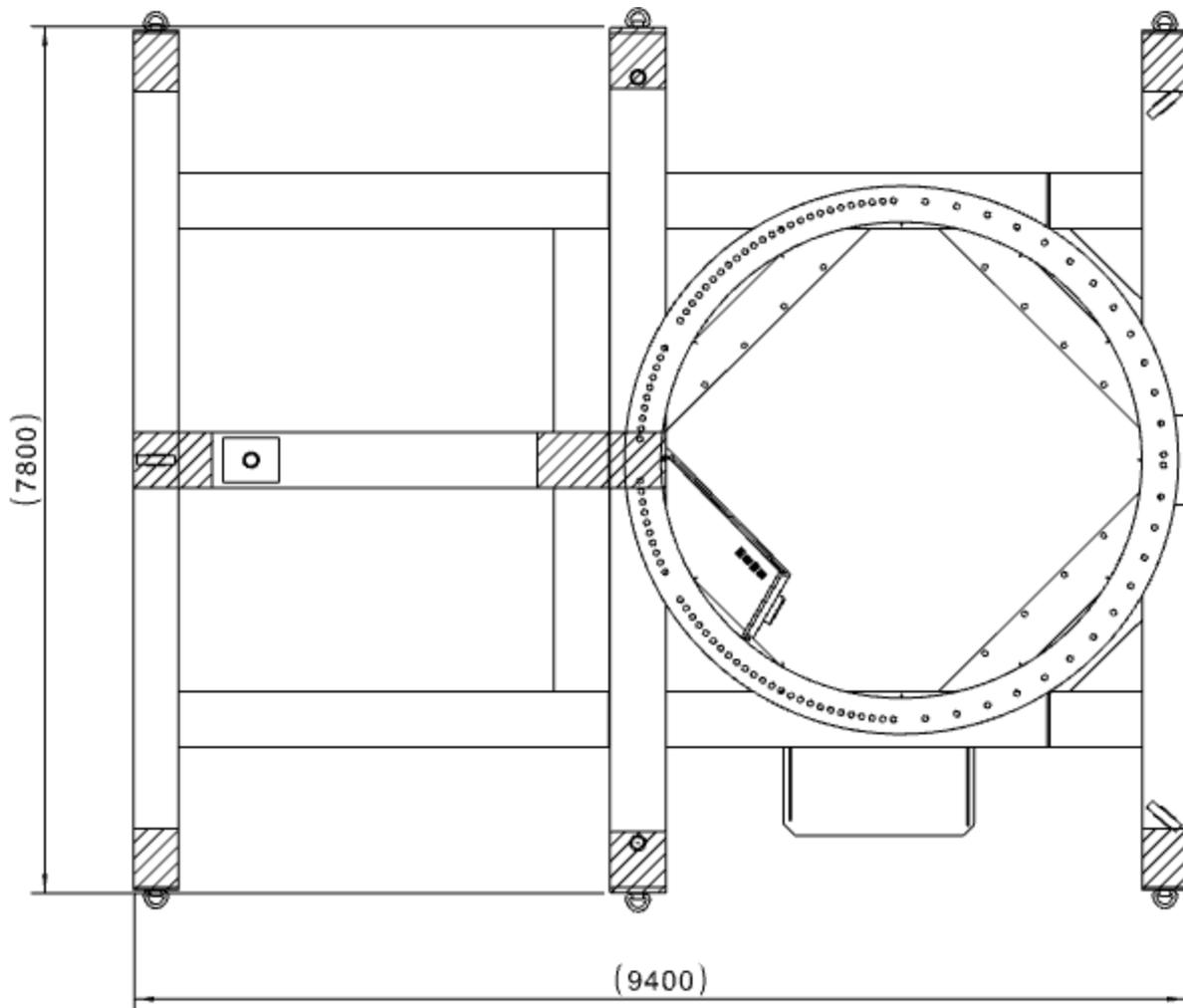
**Figure 5-7 – Overall dimensions – strong points on example nacelle frame**
