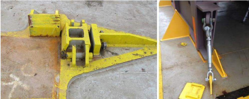
**Figure 5-3 – Corner stoppers and lashing options on nacelle transport frame example**
