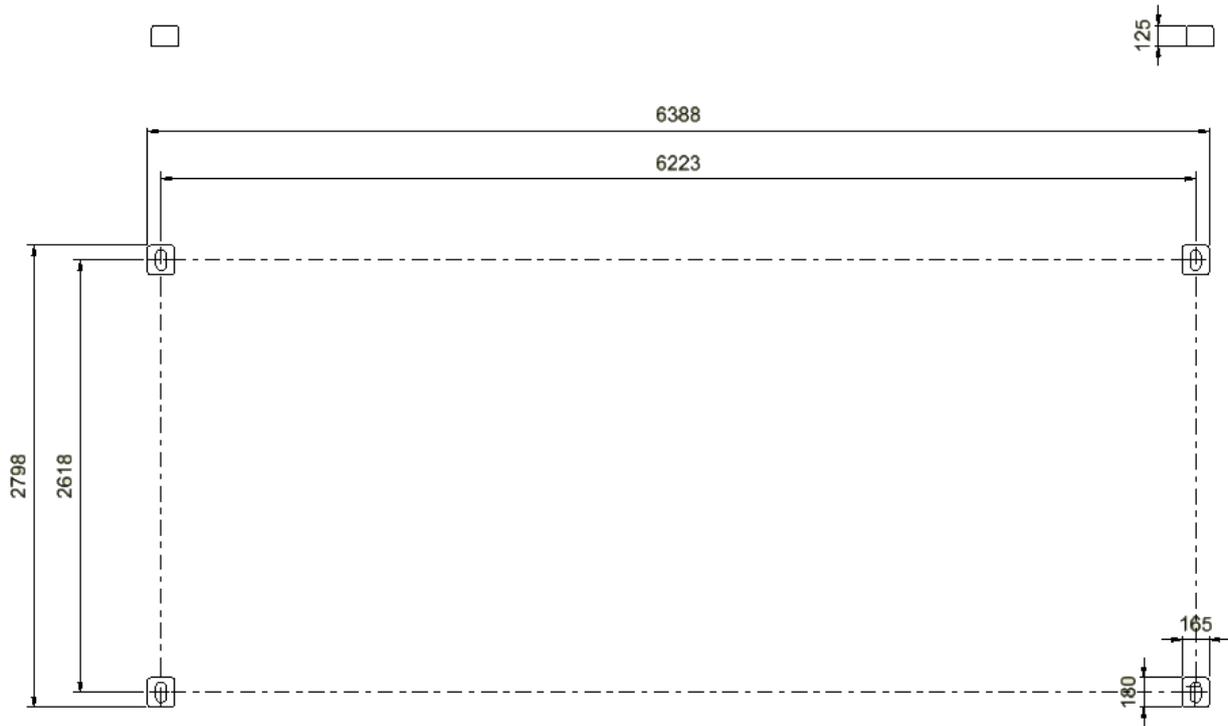
Figure 8-1 – Schematics of 20ft container corner casting footprint.
