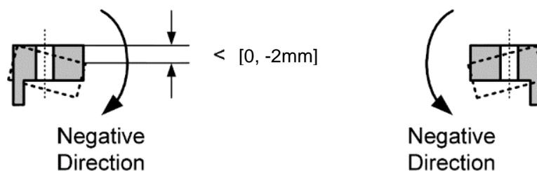
Figure 4-8 – Angular displacement definition
