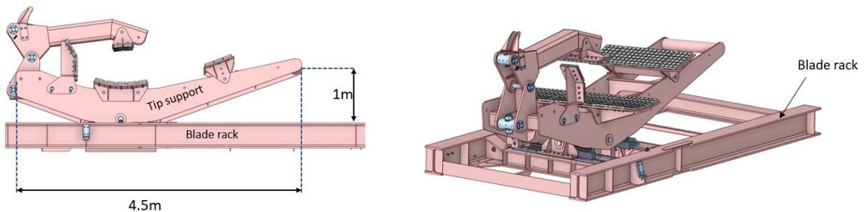
Figure 6-9 - Blade tip support interface on blade rack example
