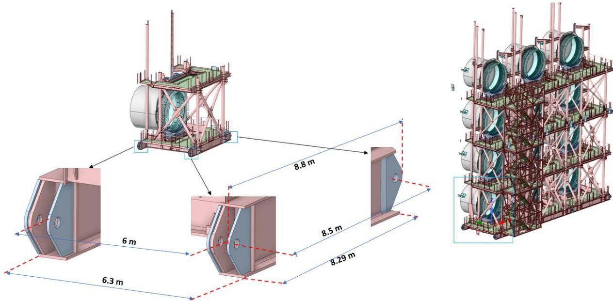
**Figure 6-13 – Modular connection between modules of the root end blade rack example**
