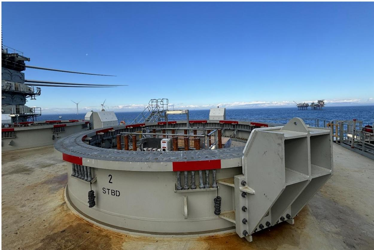
**Figure 4-5 - Tower adapter example**
