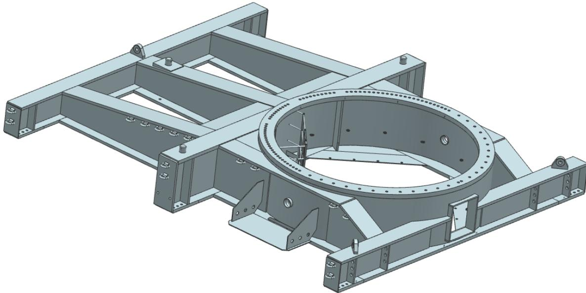
Figure 5-1 - Nacelle transport frame example
