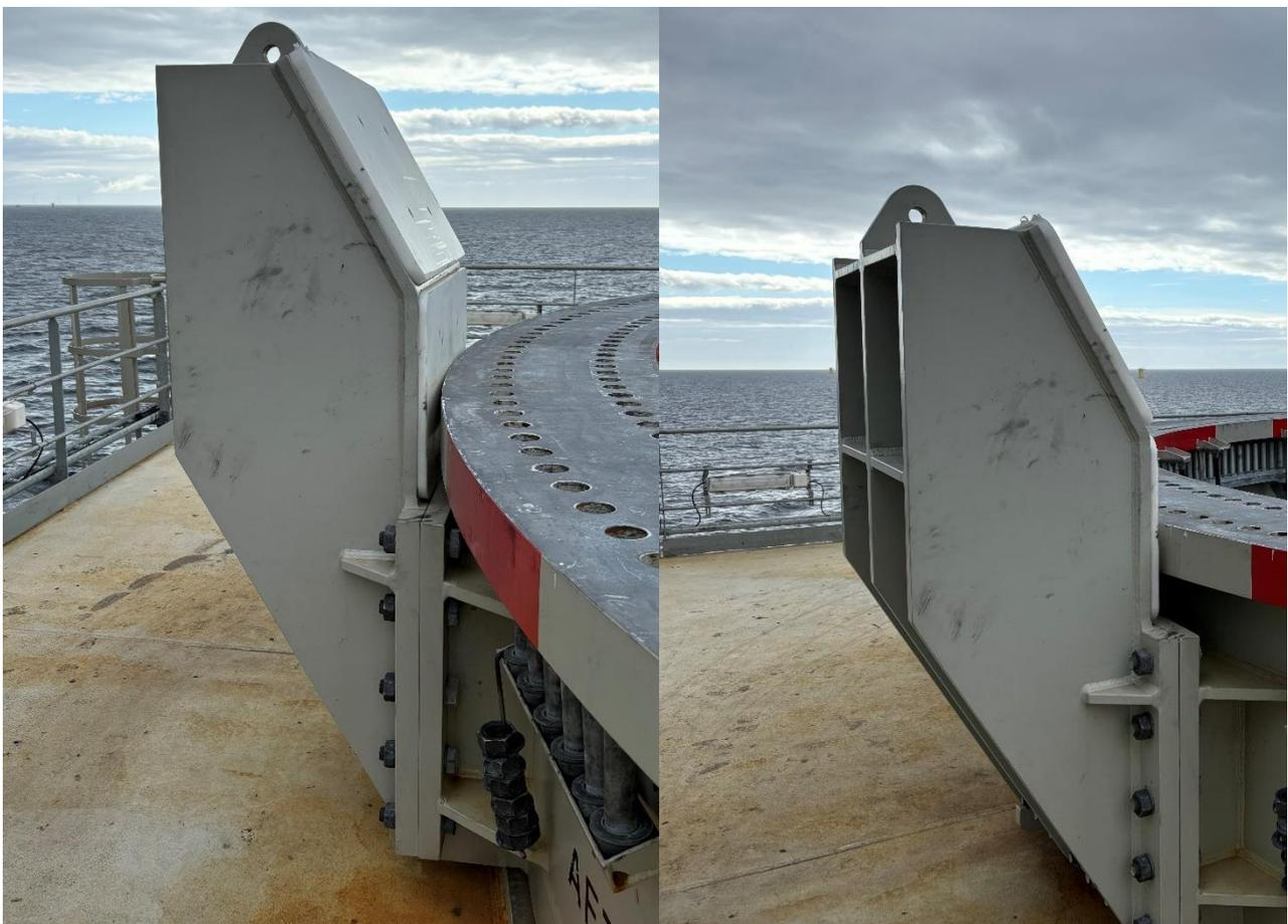
Figure 4-9 - Tower Sea fastening bumpers example
