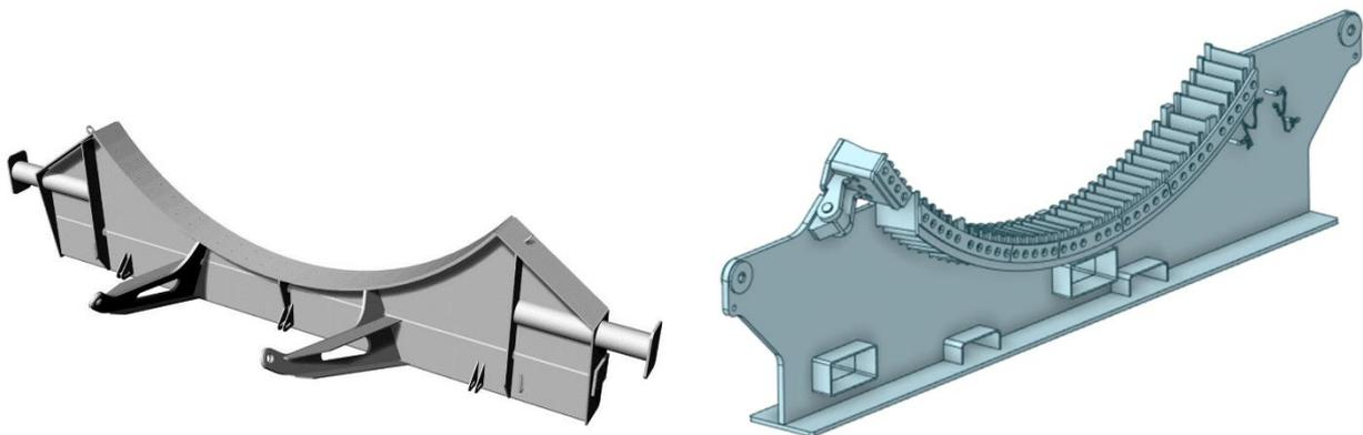
**Figure 6-7 – OEM-specific root end blade foot interface examples**
