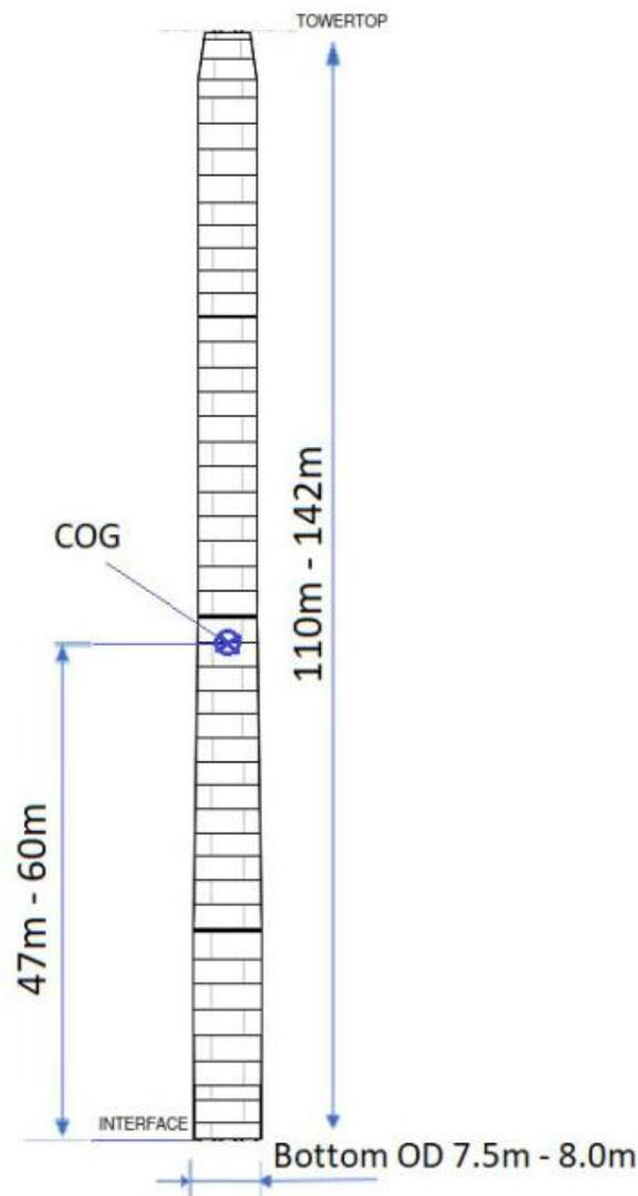
Figure 4-1 – Schematic of tower CoG
