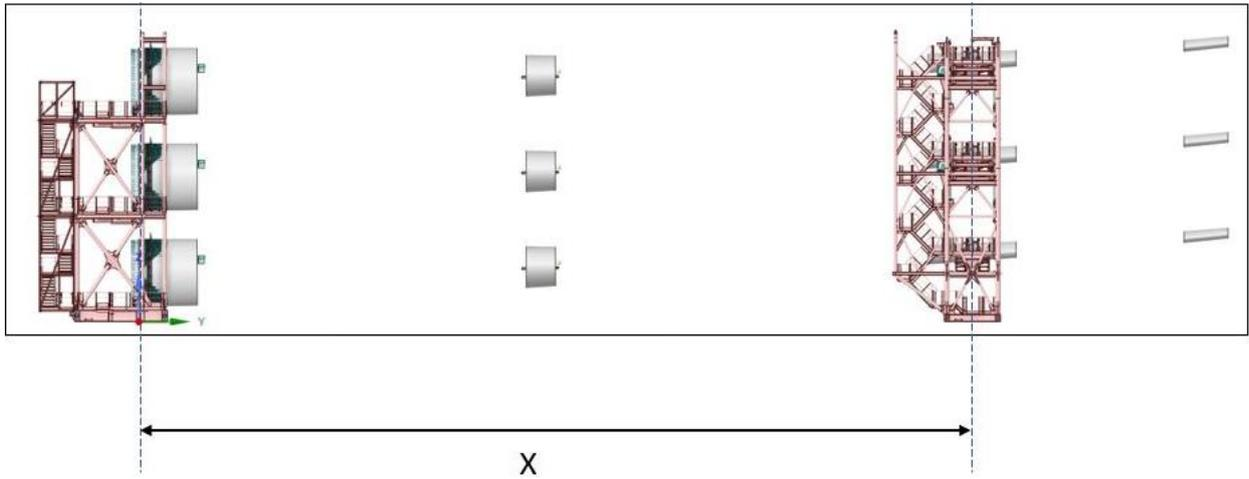
Figure 6-5 - Spacing between root and tip support points
