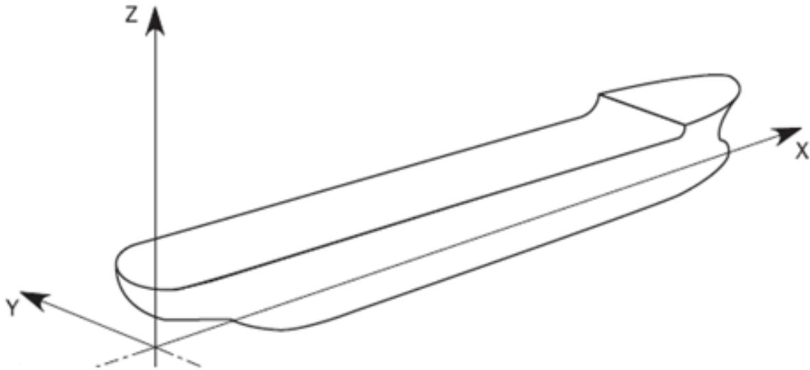
**Figure 5-2 - Vessel coordinate system**
