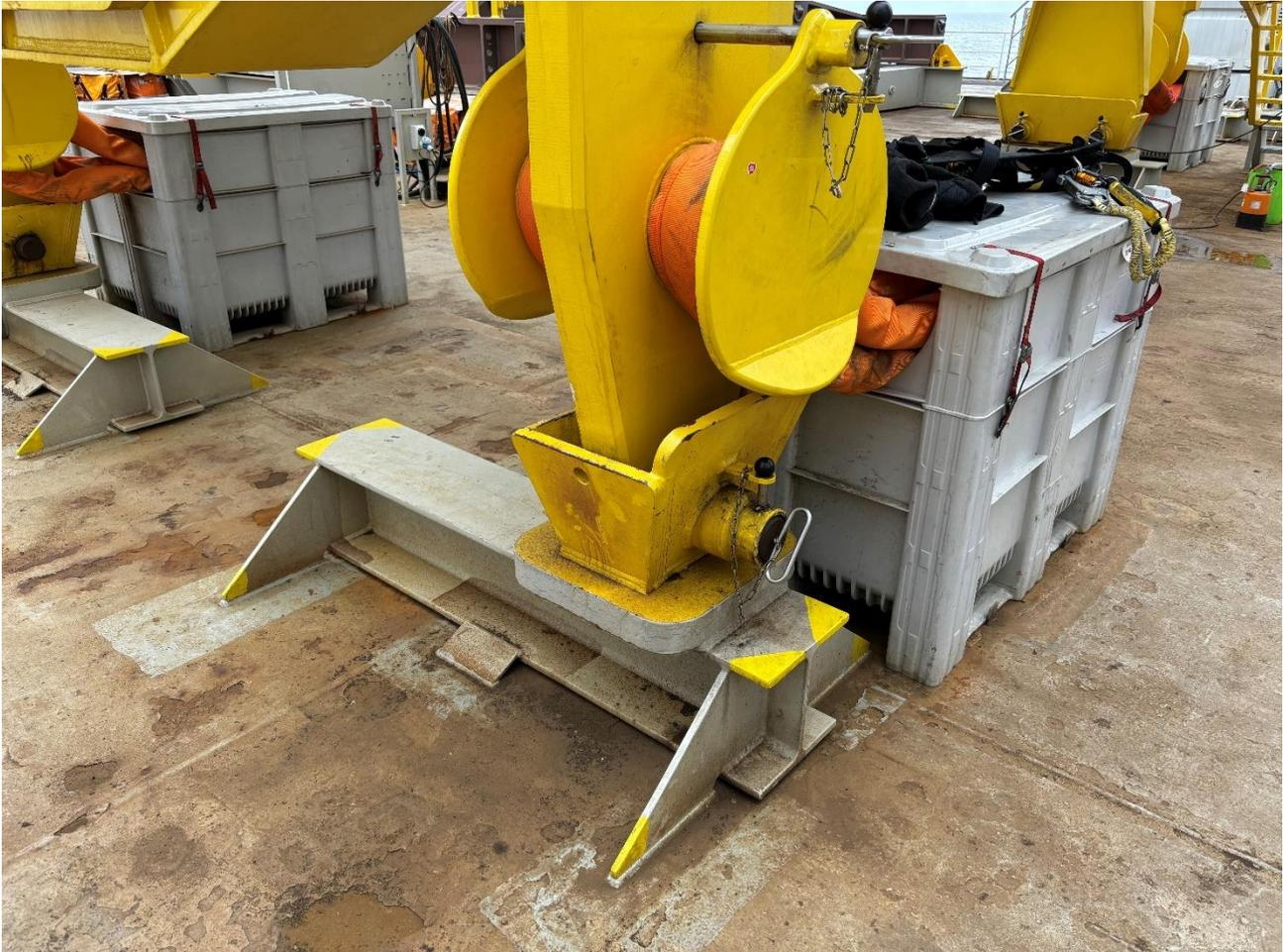
**Figure 7-2 - Nacelle yoke support example**
