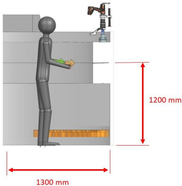
Figure 4-6 - Working height requirement for tower adapter
