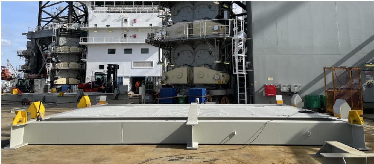
**Figure 5-5 - Deck beam reinforcement example**
