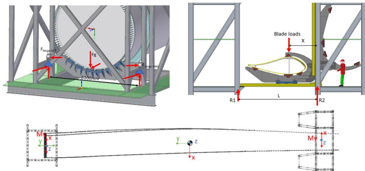
Figure 6-1 - Load points for root end (top left) and tip end (top right) blade supports, blade coordinate system aligned with vessel coordinate system (bottom)
