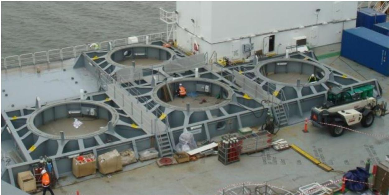
Figure 4-2 –Tower seafastening example
