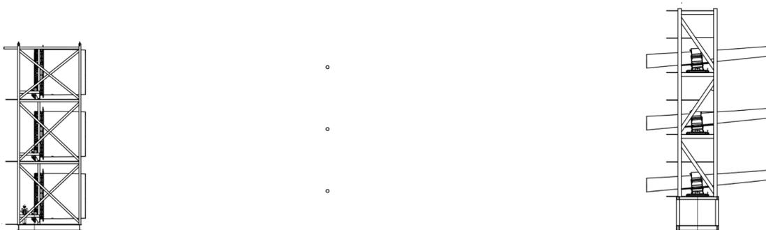
**Figure 6-4 – Example of blade seafastening, side view**
