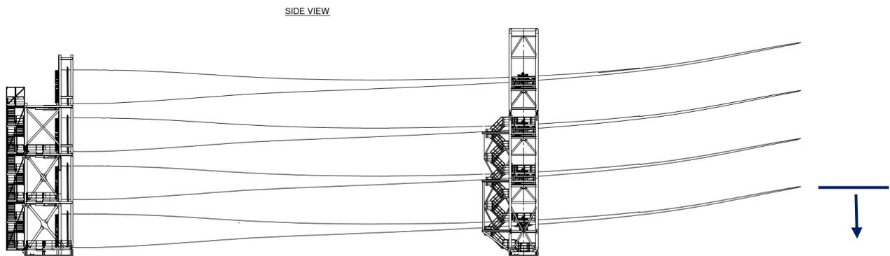
**Figure 6-14 – Direction of blade tip deflection for an example blade rack arrangement**
