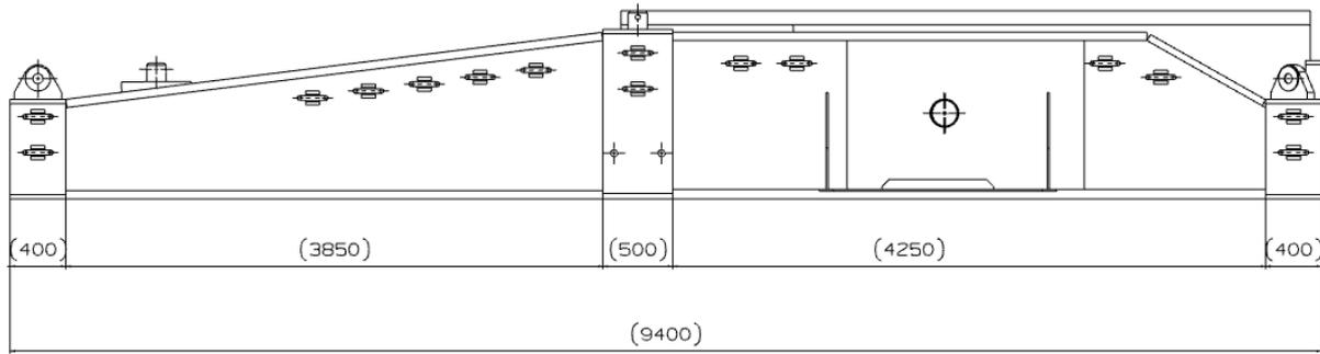
**Figure 5-6 - Overall dimensions of an example nacelle frame**
