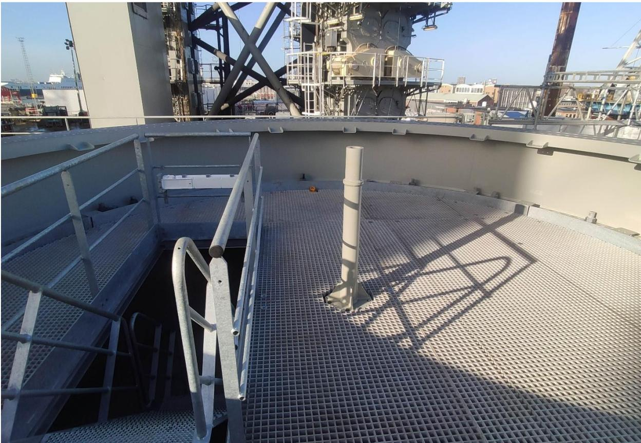
**Figure 4-4 – Grating inside tower seafastening example**
