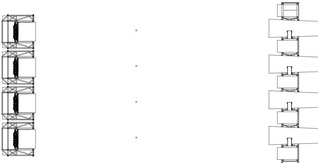
**Figure 6-3 – Example of blade seafastening, top view (4 root modules and 5 tip modules shown)**
