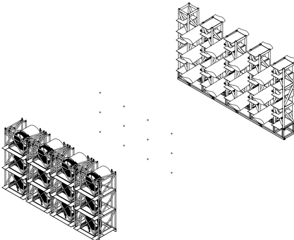
Figure 6-2 – Example of blade seafastening
