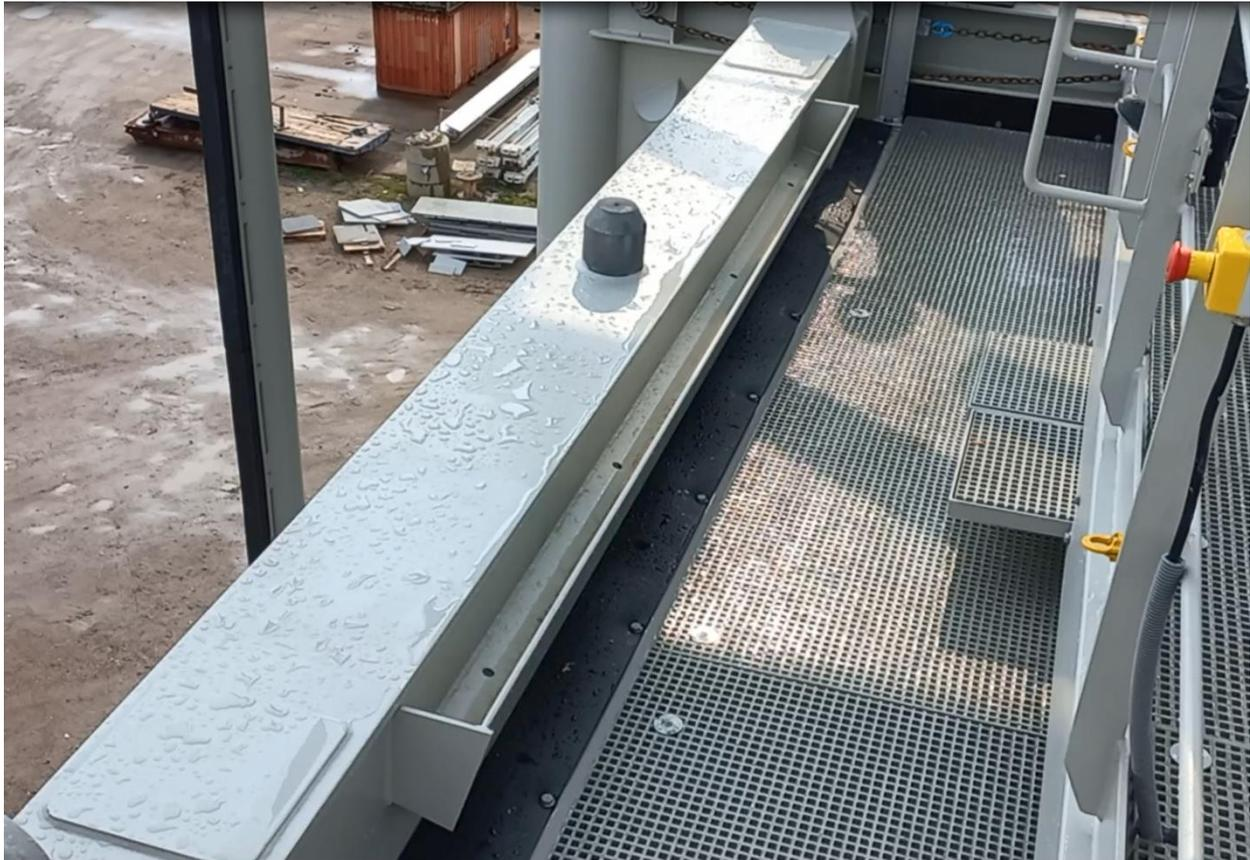
Figure 6-8 - Blade foot mounting interface on the blade rack (for root end) example
