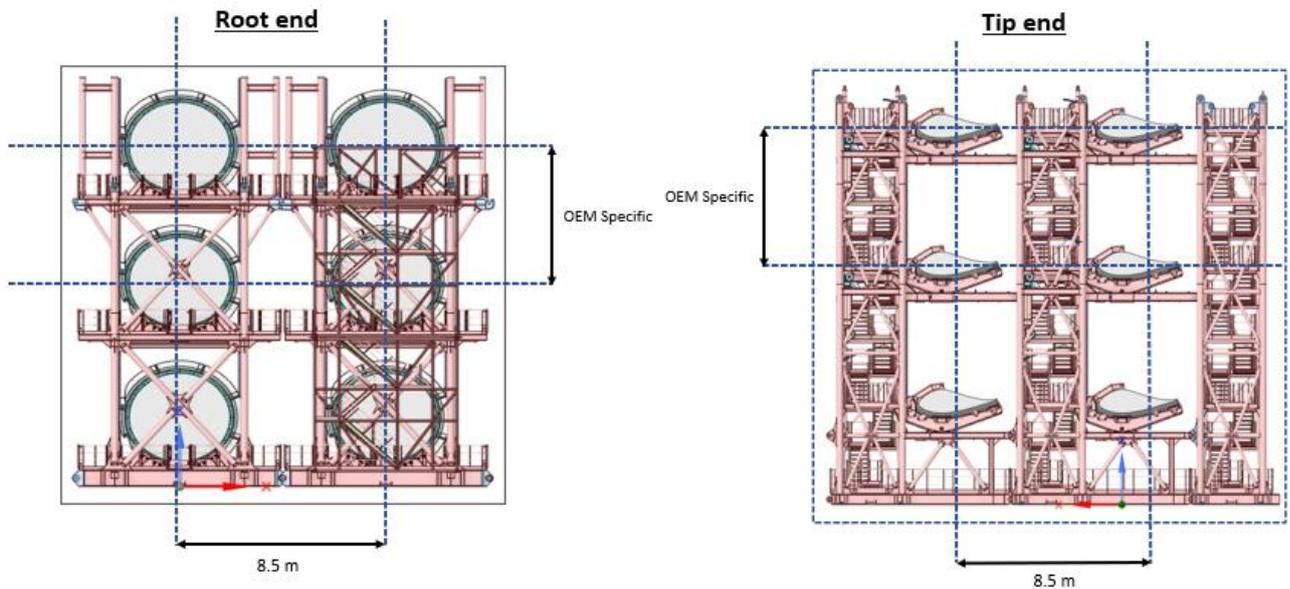
**Figure 6-6 – Blade “Centre-to-Center” distance (common for B108, B115, and V236 115.5m)**
